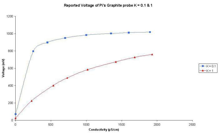
If the water has a moderate conductivity, it is best to use a probe with a K value of 1 (red line on the graph). Although it doesn't have high response the K=0.1 probe has in low conductivity solutions, it instead has a constant response from low to moderate levels of conductivity and the probe is able to give an accurate reading across a wide range of conductivity values, which can be indispensable if the conductivity of a water solution is unknown.
