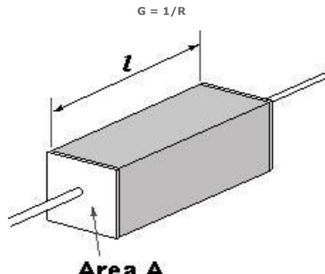
Often it is necessary to relate the conductance to a specific length of material, as well as a constant cross sectional area. This is the ratio of the distance 'l' (between the electrodes), to the area 'A' of the electrodes. The ratio of 'l' and 'A' is called the **cell constant (K)**.
