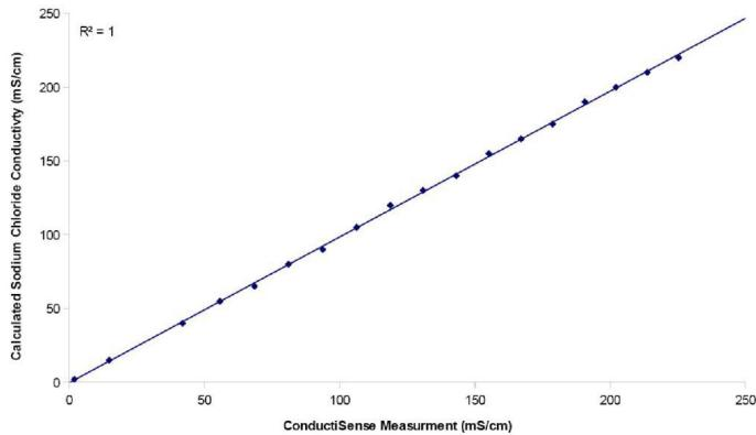
The maximum conductivity value a sodium chloride solution can produce is 230,000 $\mu\text{S}/\text{cm}$ , or 230mS/cm, before it becomes saturated solution, i.e. no more sodium chloride will dissolve no matter how much is added. As can be seen from the graph above, the toroidal probe accurately measured to this limit, and is capable of accurately measuring conductive solutions up to 2,000mS/cm, which is far beyond the range the graphite probes are capable of measuring.
